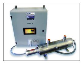
These systems are ideally suited for commercial/industrial and marine effluent applications. The Quattra UV has an automatic integrated pneumatic wiper system (external air supply required) to maintain lamp efficiency and a proprietary UV reaction chamber, designed to increase the dwell time inside the chamber. Engineered and designed to provide a very high UV dose, extended dwell time at rated flow of 50 / 100 GPM.
